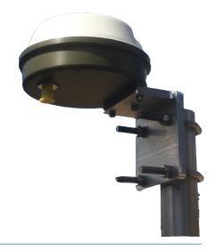
Provides superior performance for external mounting in harsh or marine environments. The radome is 4 mm GRP and the base is milled from aluminium and hard anodised giving an attractive green finish, which is mechanically resilient and resistant to corrosion.
